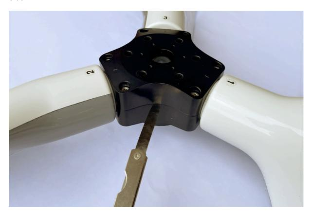
Clean the propeller surface with lukewarm water with non-corrosive detergent added.
