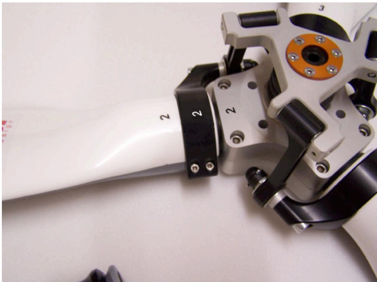
Also note that the numbers are shown on both parts of the propeller hub. The pull rods for adjusting the blade-pitch are marked by numbers too. During the assembly, these numbers MUST correspond to each other.
