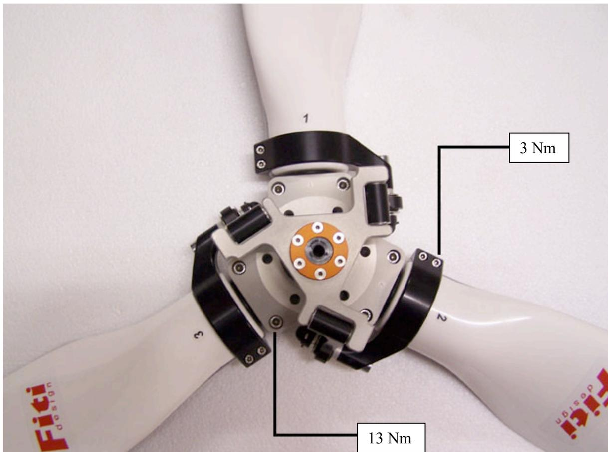
Place the assembled propeller on a level surface and adjust the pull rods and the adjusting sleeves of each blade.
