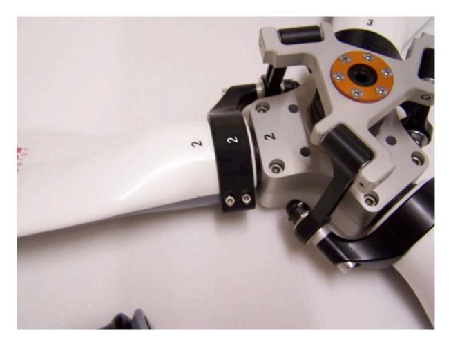
Also note that the numbers are shown on both parts of the propeller hub. The pull rods for adjusting the blade-pitch are marked by numbers too. During the assembly, these numbers MUST correspond to each other.
