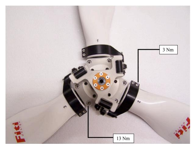
Place the assembled propeller on a level surface and adjust the pull rods and the adjusting sleeves of each blade.
