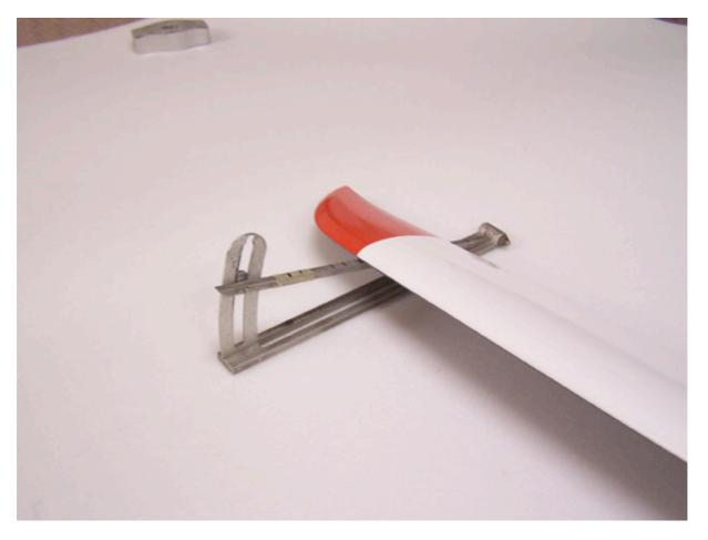
Measuring is performed on the boundary of the red and white color. Rotax 912  $80 \text{ HP} - 17^{\circ}$ Rotax 912  $100 \text{ HP} - 19^{\circ}$
